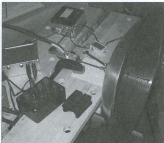
Fig. 5 24 GHz assembly with mixer head, LO and fruit bowl dish
