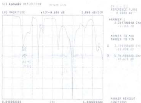
Fig.: Measured return loss of HB9MPU multiband feed
