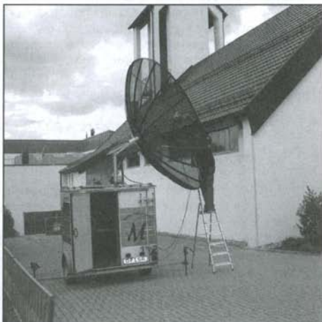
The HB0/DF1SR 3m mobile dish for 23 and 13cm EME in May 2008
