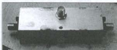
Fig. 4 Housing of the 24 GHz mixer head - bottom side, looking at the IF jack
